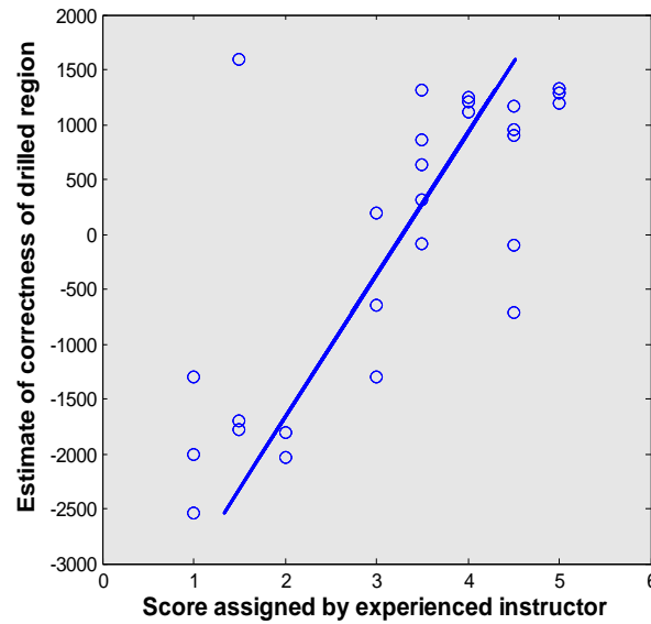
Figure 21. Relationship between expert-assigned scores (x axis) and estimate of drilled region correctness (y-axis), along with a linear fit ( R=0.76 , p<0.001 ). Each dot represents one pass through the simulated procedure by one subject. The strong correlation supports the validity of our drilled-region-correctness estimate as an automatic performance metric.
