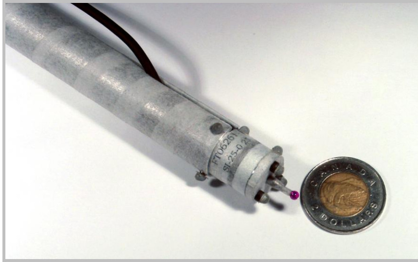
Figure 58. The sensor used to acquire force and torque information, alongside a coin to indicate scale.
