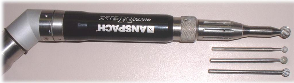
Figure 3. A typical surgical drill with an assortment of drilling burrs.
