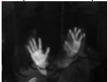
Figure 3 TouchLight image processing steps illustrated. Images are captured in an office with normal indoor lighting: (a) raw input from both cameras, (b) input after lens distortion correction, showing display geometry during calibration, (c) input after perspective correction to rectify both views to display, and (d) fused image obtained by multiplying perspective corrected images shows only the objects that are very near the display. Hand on the left is placed flat on the display, hand on the right is slightly cupped, with tips of fingers on the display, and surface of palm above the display.
